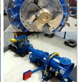
Kaplan turbines are suitable for low heads and high flow applications, with achievable efficiencies of over 92% and with grey flexibility. We manufacture vertical and horizontal axis Kaplan turbines. Fixed, single or double regulation for the best flexibility is available. We offer proven technology.
